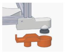
Place the pins that serve as a stop to the leading edge of the wing in its position
