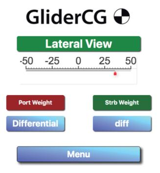
The numbered rule in the upper part will help us to identify in a simple way the weight deviation between both sides
