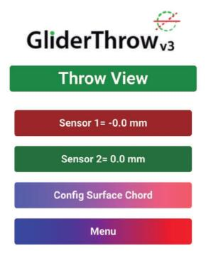
Here you can see the throws, in mm, calculated with Chords stored in the units, according to this diagram.
