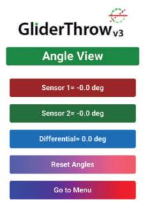
In this Screen you can check the reading of both sensors and perform any adjustment in your plane for instance if your reference information is in degrees or if you want to do so.
