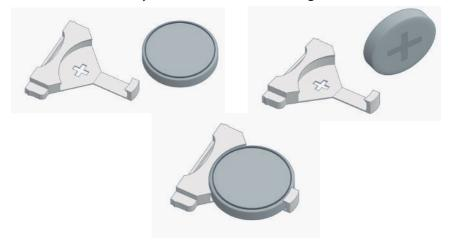
Additionally, the tray incorporates a projection in such a way that it can only be inserted back into the slot in one position.
