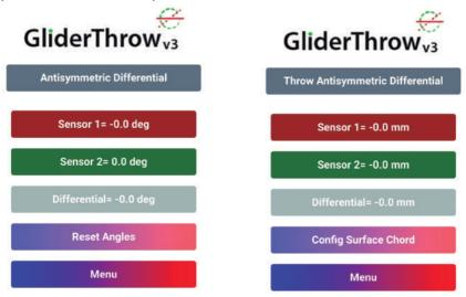
When you are trimming or calibrating a Symmetric Flight Control, like the flaps you want both sides control surfaces deflect the same: Symmetry in an airplane is critical for stable flights... Then the standard page is ideal it will show the difference in reading of the two sensor: Remember sensor 2 minus sensor 1.
