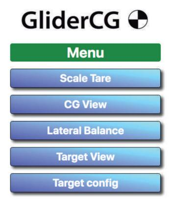
The first menu option "Scale Tare" allows you to zero the weight measurement or tare the scale.
