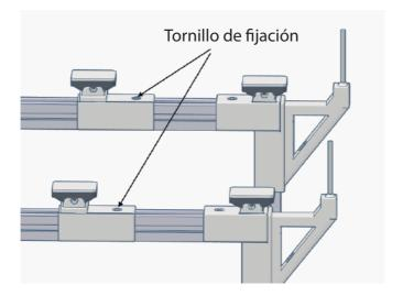
If, during the use of the GliderCG Scale, you wish to vary the distance of the supports to change between different models, once the distance has been modified you must perform a tare of the device as explained below.
