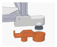
Insert the arms into the base and verify that the front pins are in the front position (towards the power button). Place the pins that serve as a stop to the leading edge of the wing in its position
